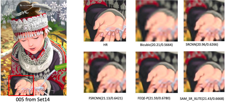
Fig. 6. Qualitative comparison on Set14 [43]. SAM_SR_XLITE outperforms bicubic interpolation, SRCNN [7] and FSRCNN [8] and on par with FEQE-P [40], while being 4 – 6 \times smaller in operation size.
